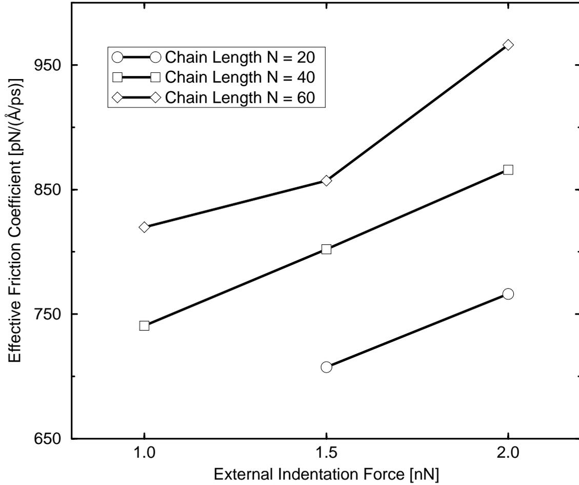
FIG. 5. Force dependence of the effective resistance coefficients. The result for  $N = 20$  and  $F_{\text{external}} = 1.0$  nN is spoiled by finite chain length effects and omitted from the plot.
