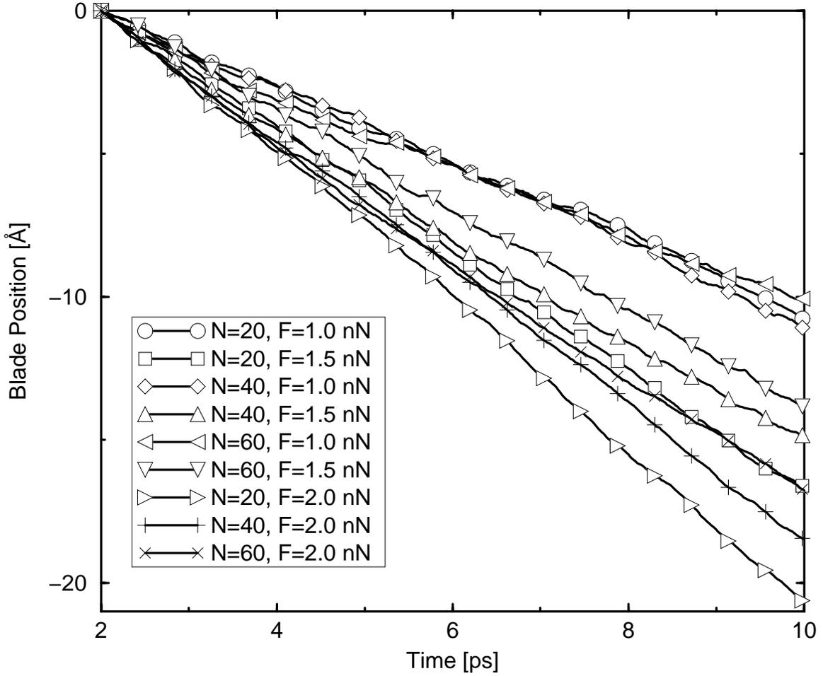
FIG. 3. Tool indentation curves for chain length  $N = 20, 40,$  and  $60,$  and indentation forces  $F_{\text{external}}$  of  $1.0, 1.5,$  and  $2.0$  nN.
