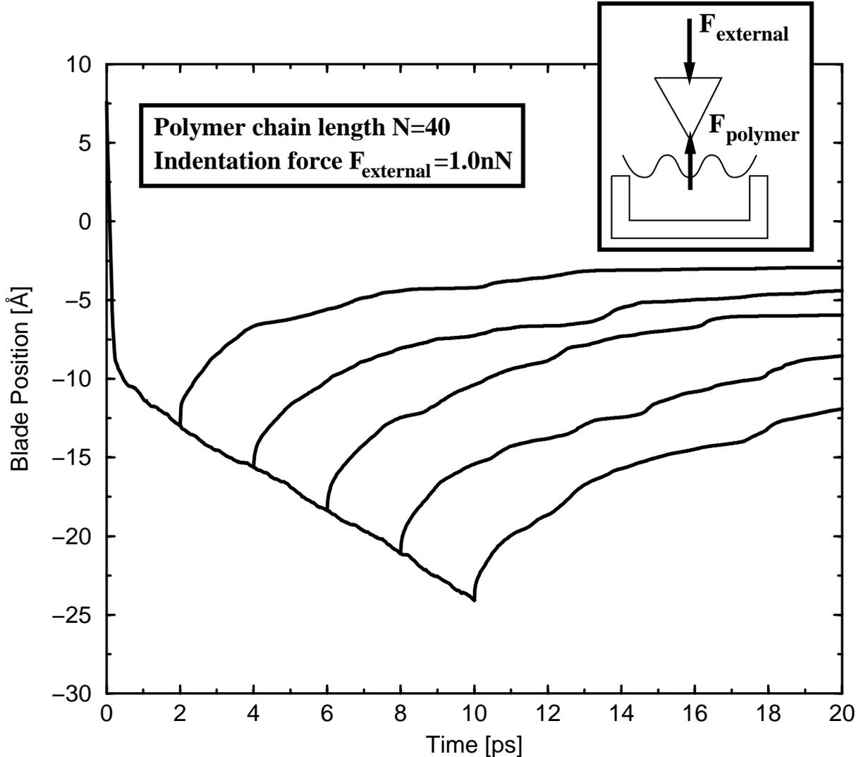
FIG. 2. Indentation and free drift curves with chain length  $N=40$  and indentation force  $F_{\text{external}} = 1.0$  nN. During the indentation process, both  $F_{\text{external}}$  and  $F_{\text{polymer}}$  are different from zero. For the free drift experiments,  $F_{\text{external}}$  has been set to zero.
