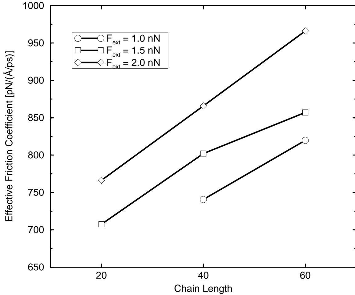
FIG. 4. Chain length dependence of the effective resistance coefficients. The result for  $N = 20$  and  $F_{\text{external}} = 1.0$  nN is spoiled by finite chain length effects and omitted from the plot.
