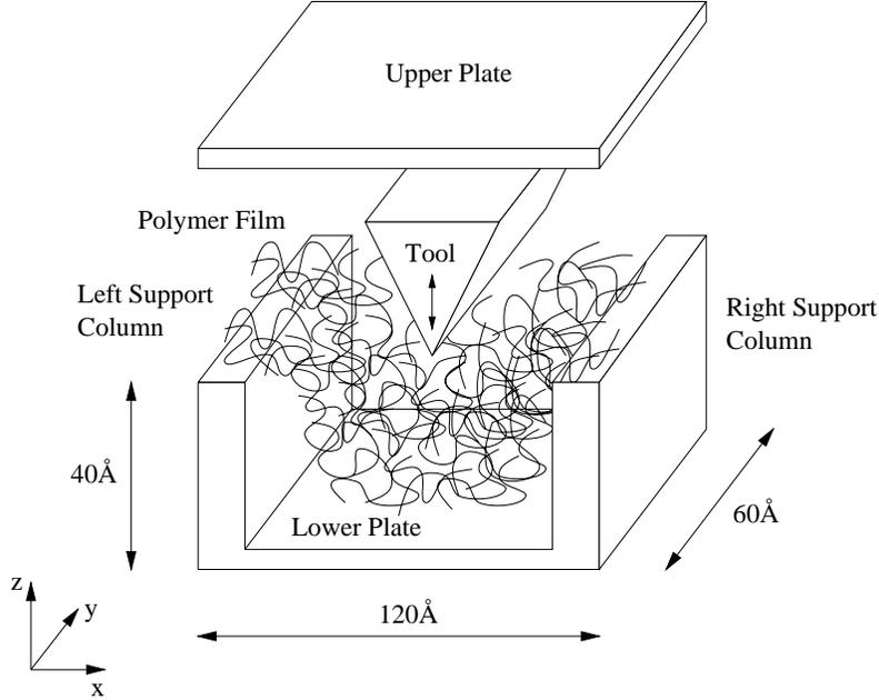
FIG. 1. Sketch of the blade indentation experiment (lengths in Å).
