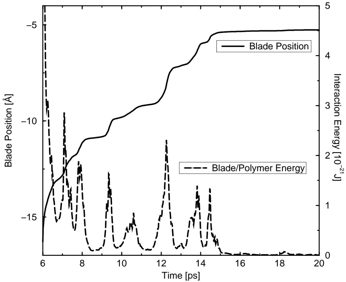
FIG. 7. Free drift dynamics of a single polymer configuration. Shown are the blade position and the tool/polymer interaction energy.
